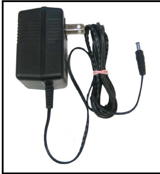
Figure 1. Typical “Wall Wart.”
